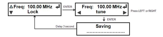
By pressing the ENTER push button, you can modify the set frequency using the RIGHT (the frequency increases) and LEFT push buttons. After having set a new frequency value, press the ENTER push button to confirm the choice. The exciter will release from the current frequency and it will latch onto the new operating frequency.
