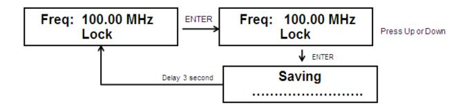
By pressing the ENTER push button, you can modify the set frequency using the UP (the frequency increases) and DOWN (the frequency decreases) push buttons. After having set a new frequency value, press the ENTER push button to confirm the choice. The exciter will release from the current frequency and it will latch onto the new operating frequency.
