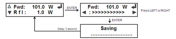
To increase the level, press the RIGHT push button and to reduce it, press LEFT. As the set level increases or decreases, the bar becomes longer or shorter to display the current setting. When the designed level is reached, press ENTER to confirm and exit the predefined menu.
