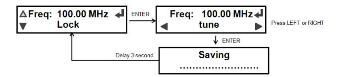
By pressing the ENTER push button, you can modify the set frequency using the RIGHT (the frequency increases) and LEFT push buttons. After having set a new frequency value, press the ENTER push button to confirm the choice. The exciter will release from the current frequency and it will latch onto the new operating frequency.
